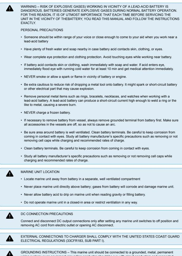
GROUNDING INSTRUCTIONS – This marine unit should be connected to a grounded, metal, permanent wiring system; or an equipment-grounding conductor should be run with circuit conductors and connected to equipment-grounding terminal or lead on unit. Connections to unit should comply with all local codes and ordinances
