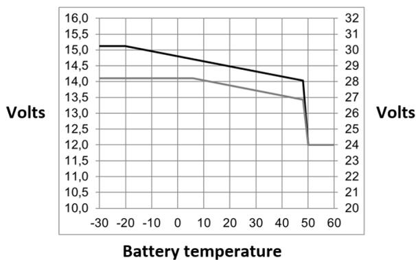
Default output voltages for Float and Absorption are at 25 °C for 12V or 24V battery bank, to arrive at 48V battery bank voltages, multiply the 24V voltages by a factor two.
