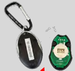
Hand-held Remote Start/Stop Keyfob (front view)
