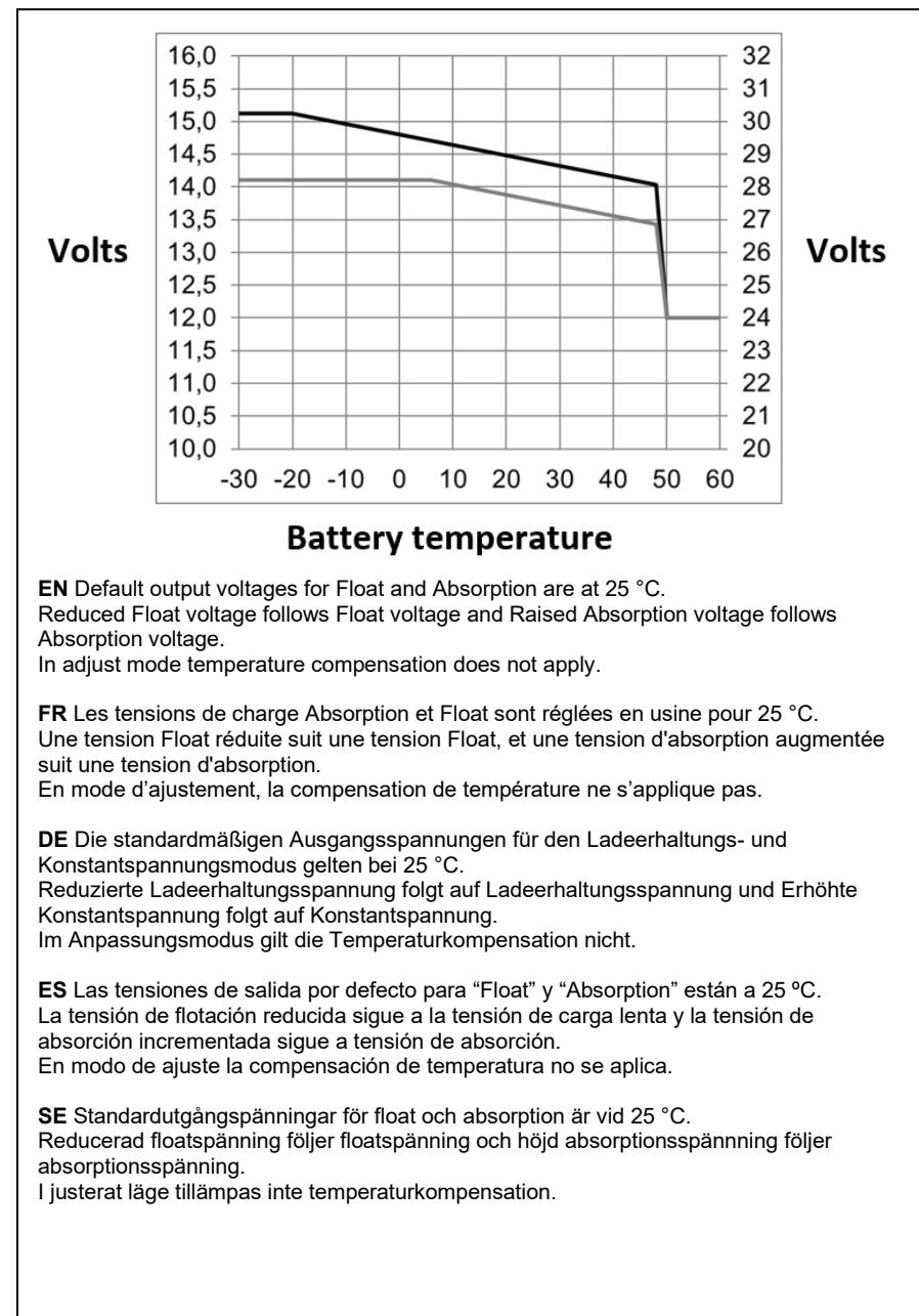
**EN** Default output voltages for Float and Absorption are at 25 °C.
