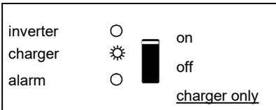
The AC input voltage is switched through and the charger operates in float mode.
