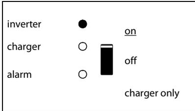
The inverter is switched on and supplies power to the load. Battery operation.
