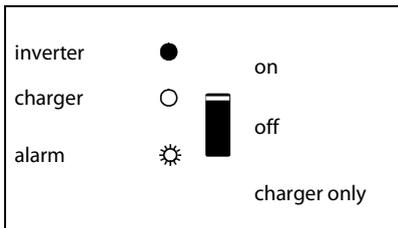
The inverter is switched on and supplies power to the load.
