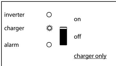
The AC input voltage is switched through and the charger operates in float mode.
