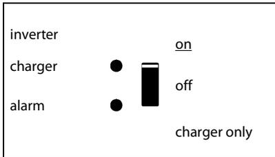
The AC input voltage is switched through and the charger is switched off.
