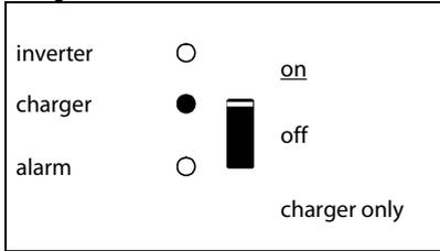
The AC input voltage is switched through and the charger operates in bulk or absorption mode.
