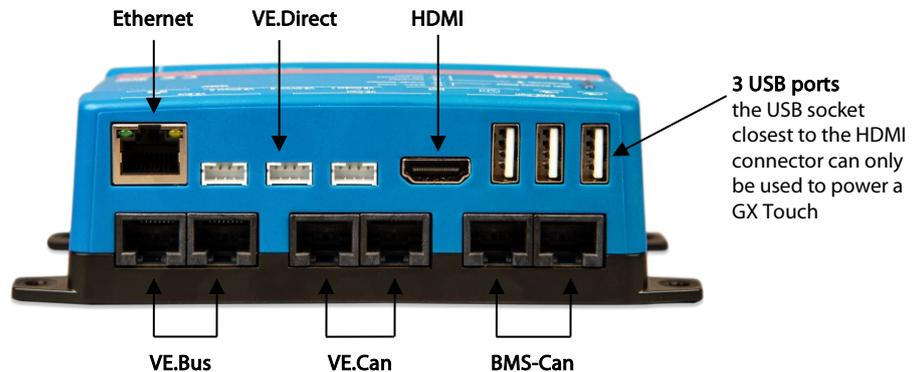
3 USB ports the USB socket closest to the HDMI connector can only be used to power a GX Touch
