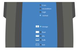
4. Select the charge mode and charge current limit most appropriate for the battery type and capacity.
