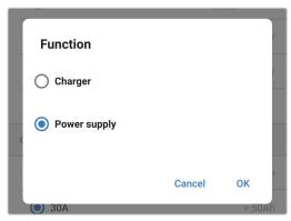
After a short delay the BULK, ABS, FLOAT and STORAGE LEDs will be illuminated to indicate the charger function has changed to Power supply mode.
